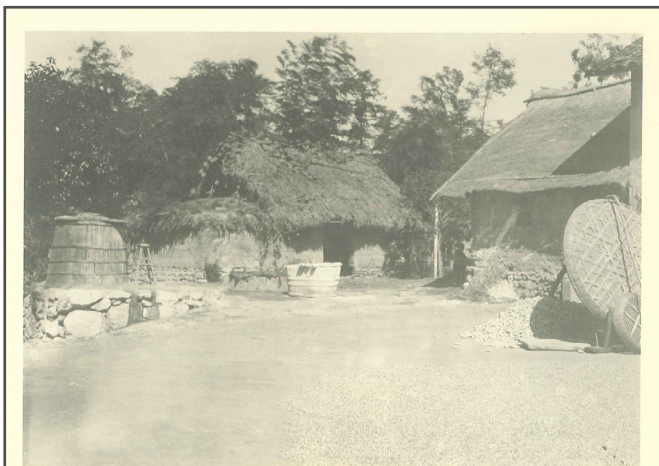
Fig. 10. Pulp materials are sometimes digested by boiling with various reagents, in wooden vats like the one shown at the left in the photo above. A lime tub is seen in the background.
